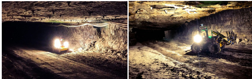
Fig. 1: Ground robots using LION to explore the Arch Coal Mine (West Virginia, USA), at approximately 275 meters (900 feet) underground.
